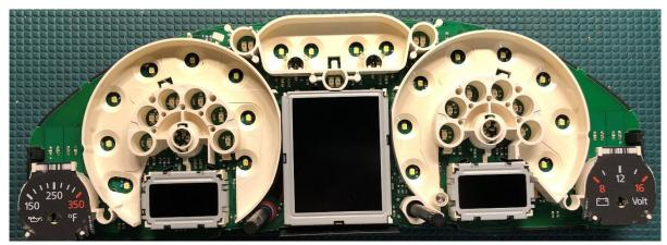
Remove the white plastic light shroud. There are hooks that need to be pressed on the backside of the PCB to release it. The odometer reset knob will also need to be pressed through the PCB by pushing in the hooks on it and feeding it through.
