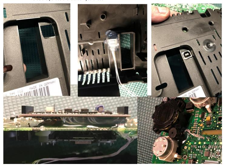
Use a rotary tool to trim an opening in the white plastic shroud to fit the ColorMFA screen. It is necessary
