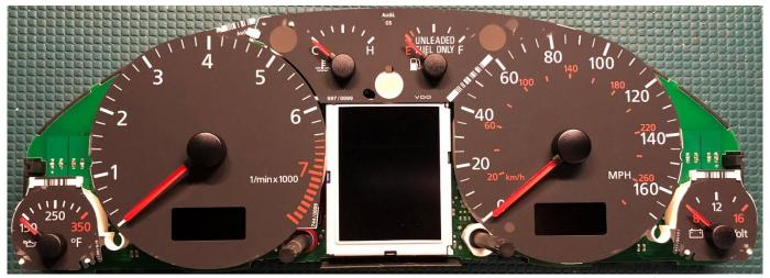
o Remove the needles by twisting counter clockwise while pulling up then remove faces.
