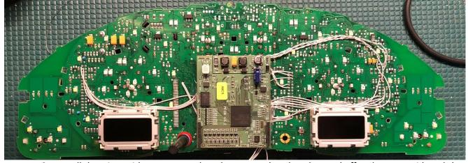
Secure all the wires with tape, epoxy, hot glue, etc so that they do not chaff and cause accidental shorts.
