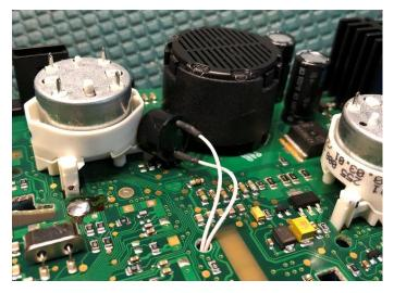
Do 1 final check with the meter to ensure each wire from the ColorMFA board is in the correct location. The solder portion is now complete.
