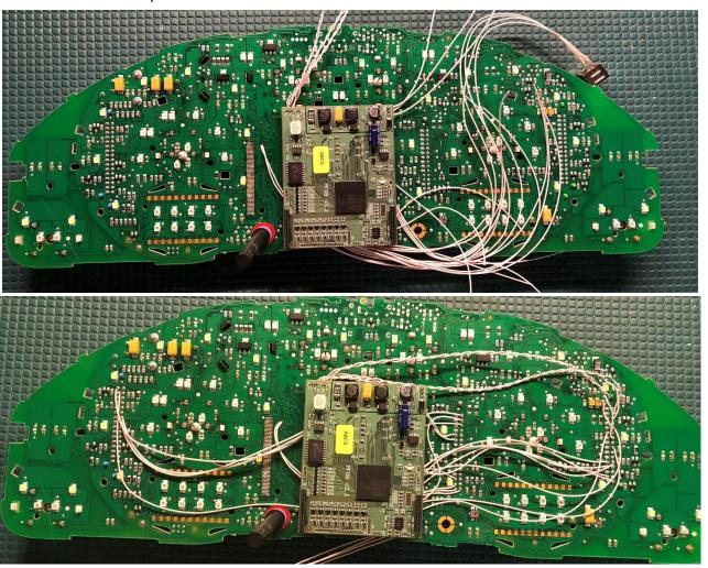
Route the 2 remaining wires for the beeper through the opening next to the stock LCD solder pads and solder them to the beeper. The longer leg of the beeper is positive. Add heat shrink to these solder joints.
