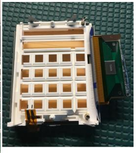
• Remove all the LED's originally behind the LCD. These LEDs do not require jumper resistors. Leave them "open". Ensure solder is not bridging any of the pads together.
