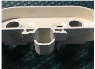
O Cut off the high beam alignment pin.
