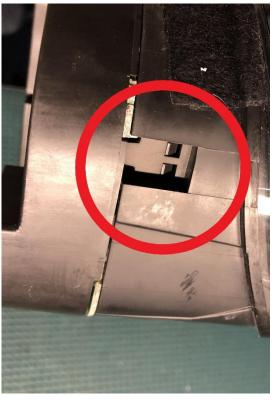
Remove back plastic housing. This is held onto the PCB with 1 hook on the far left and 1 hook on the far right.
