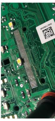
The 2-wire sensor and the plastic housing/shroud needs removed. Remove the LCD housing (2 large metal pins. Heat with solder while pulling the housing off the PCB) then located the 2 pads for the sensor and heat those up while pulling the sensor cable off.
