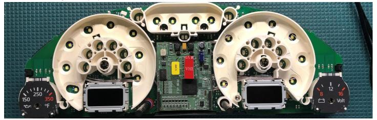
Install the ColorMFA screen onto the ColorMFA PCB. It's recommended to add about 3 layers of the double sided tape to hold the screen and board securely together. Do not stack too much tape though that it causes the screen to site above the white plastic and thus would cause the faces to not sit flush.
